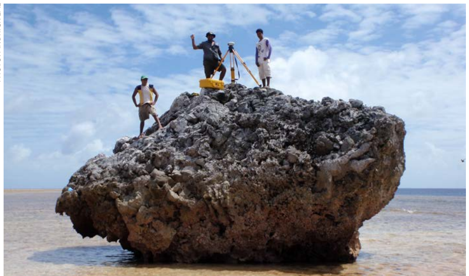
PACIFIC ISLANDS: GPS for defining territorial sea baseline on the Gilbert Islands of Kiribati.
